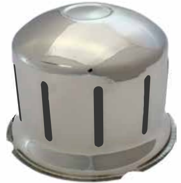
Art. 31135122 Rear axle cover for 22.5” wheels Diameter 250mm, height 165/210mm (for mounting, use mounting ring art. 31135223) € 55,00 excl. VAT / € 66,55 incl. VAT
