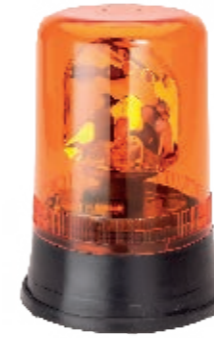
AEB "595" BEACON LIGHT 24V Amber lens, height 220mm, Ø 160mm 3-bolt mount, H1-light not included Art. 46355950 € 59,00 excl. VAT / € 71,39 incl. VAT
